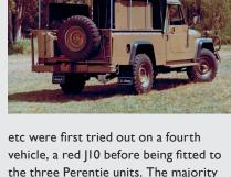
the three Perentie units. The majority of parts were sent from the US as they already had components available including harnesses and distributor shielding kits. The three Jeeps were fitted with roll bar, front electric winch, special alternator for radio equipment, long range fuel tank mounted under the tray behind the cab, jerry can holders built into the tray, rifle holder behind the seats, axe and shovel brackets and a map reading lamp on the dash.
