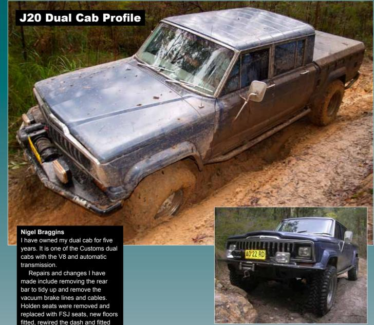
fitted, rewired the dash and fitted a stainless steel overlay. I also made a new glove box inner, fitted a radio, UHF and Hurst shifter. The canopy that was fitted to the Customs dual cab was removed.
